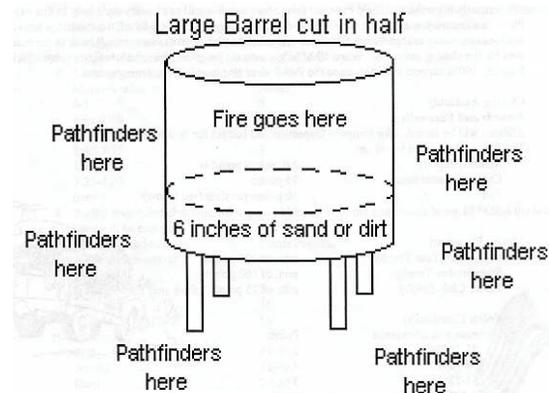
There are a number of drawbacks to using this design. If not properly cut the edge could be very sharp, and also it will have a tendency to rust over time.
