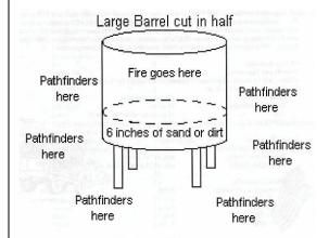
There are a number of drawbacks to using this design. If not properly cut the edge could be very sharp, and also it will have a tendency to rust over time.
